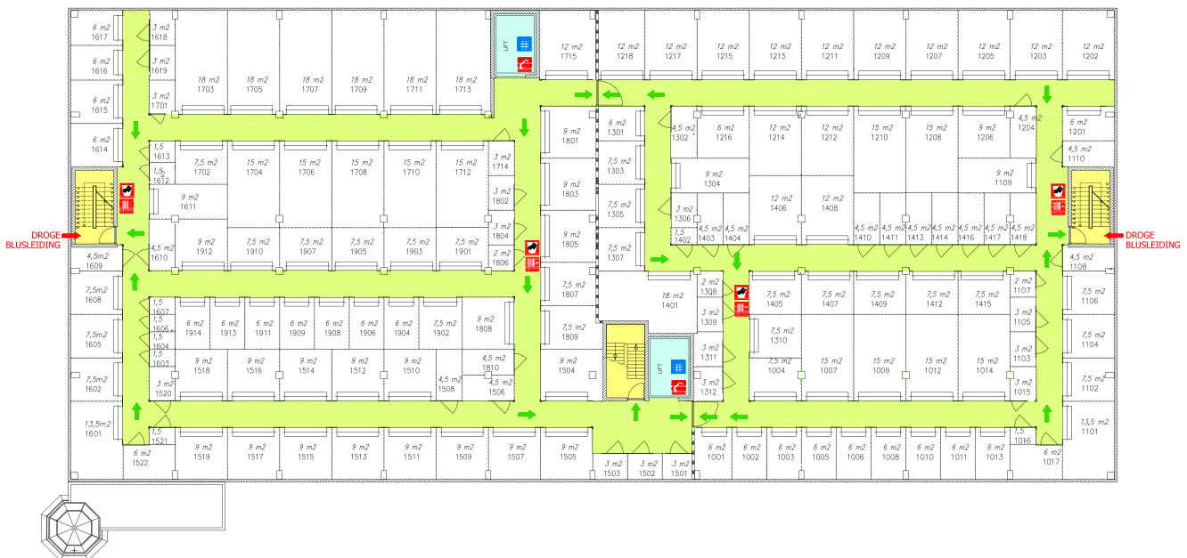
Figure 1 Typical Facility Layout (second floor) in a Self-Storage Warehouse
